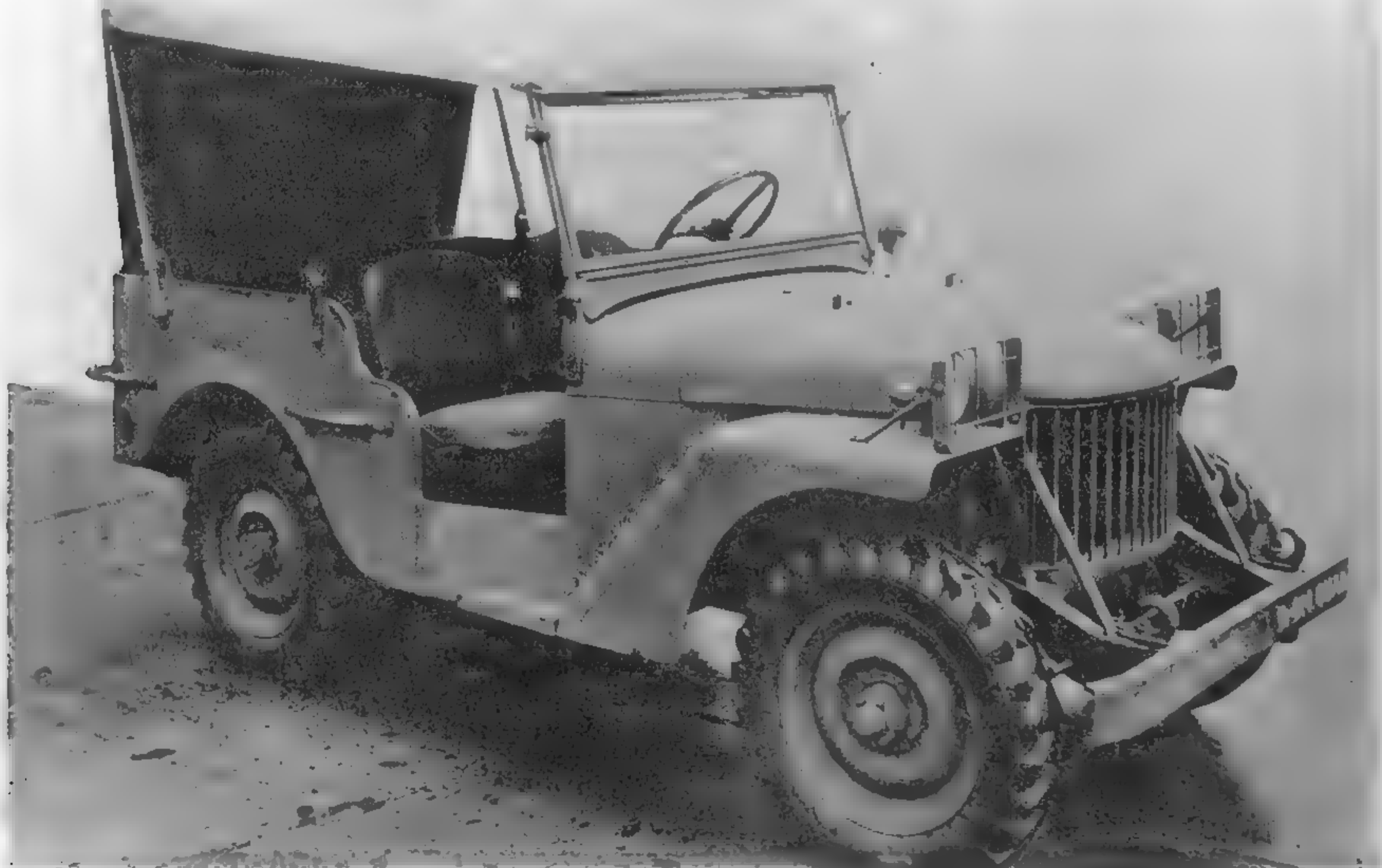
The Quad, shown here, was the Willys entry into the 1/4 ton truck competition. Notice how much the designed had to evolve to become the familiar MB. (Photo courtesy of Military History Institute)
